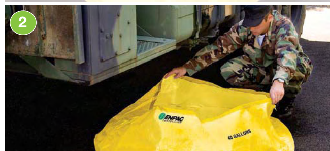
Step 2: Position pool underneath spill source.
